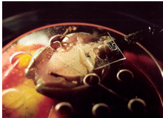
Figure 2.2: Immobilized tree frog ( Litoria caerulea ) in a petri dish with holes drilled in the bottom to expose individual toe pads which were brought in contact with the glass plate attached to the bending beam.
