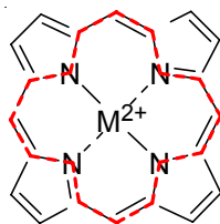
Figure 7. General structure of metalloporphyrins. The 16-membered cyclic polyene system with 18 \pi -electrons is situated along the red line.
