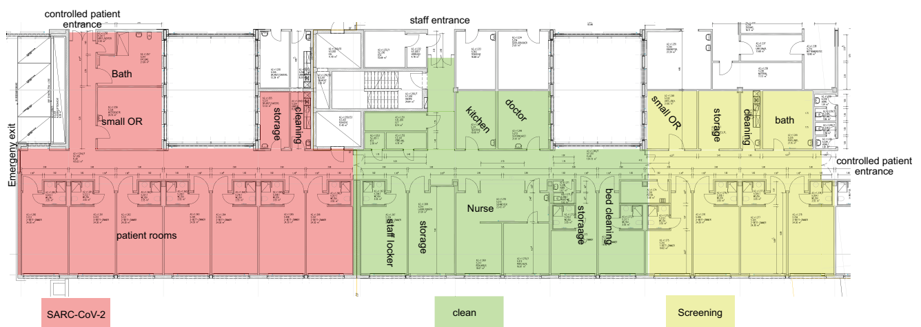
Fig. 1 Structure and structuring of the surgical SARS-CoV-2 bedside unit (modified from construction drawing of “Zentrum für Operative Medizin, University Hospital Wuerzburg”), which is divided into 3 areas: infectious area (red), for SARS-CoV-2 positive patients, potentially infectious
