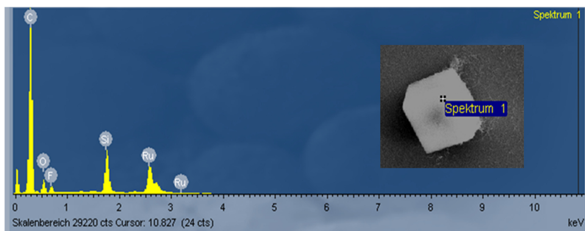
Figure S53: EDX was used to determine which chemical elements are present in the sample. EDX spectrum shows the prominent X-ray peaks for carbon (C), silicon (Si) and ruthenium (Ru). The Si peak was produced from substrate (SiO x ).
