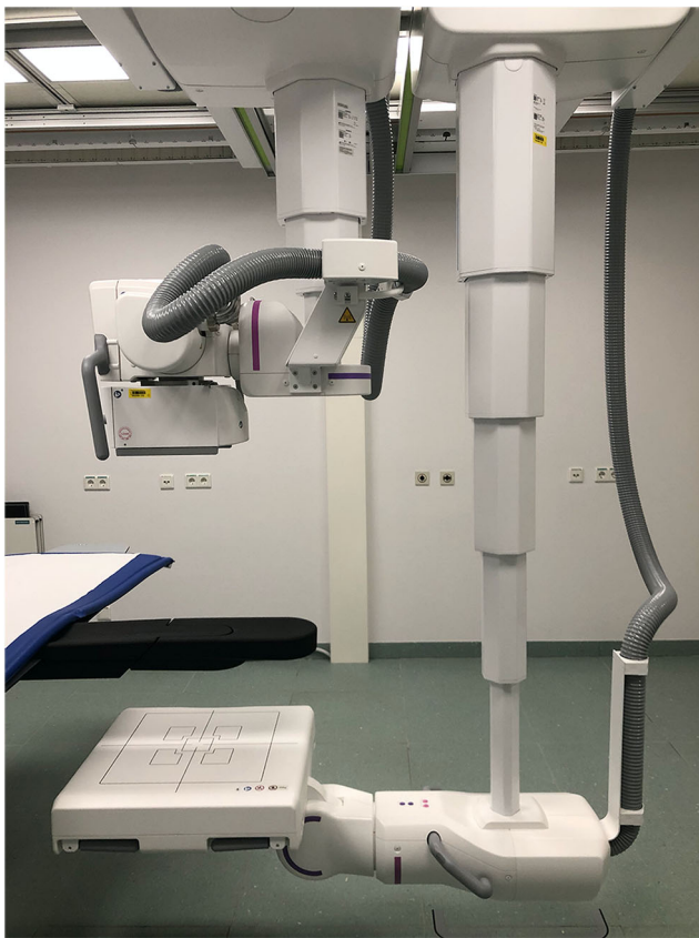
Fig. 2 Display of the tableside scan position for wrist imaging with the twin robotic x-ray system
