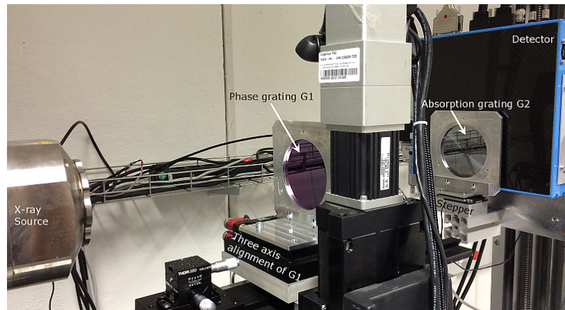
Figure 3.7: Image of the grating interferometer setup (Sub \mu ). Here the symmetric setup is shown without the G_0 grating (described in the text).
