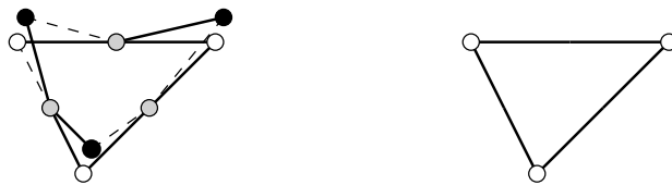
FIGURE 3.13: Tree in the auxiliary graph (left, solid lines). Its projection (right, solid lines) may contain cycles.
