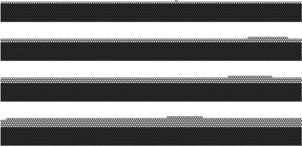
Figure 5.16: Evolution of a system simulated with zero misfit. This sequence of snapshots shows the evolution of a section of a larger system for top down number of deposited adsorbate layers 1.0 ML , 2.0 ML , 3.0 ML , 5.0 ML . The darker particles represent the substrate, the lighter particles are adsorbate particles.
