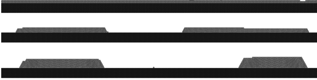
Figure 5.21: Surface topology after the deposition of 3 ML adsorbate material for different substrate temperatures with misfit \varepsilon = 2.0\% . This sequence of snapshots shows sections of a larger system for top down temperature T = 450\text{ K}, 550\text{ K}, 600\text{ K} . The darker particles represent the substrate, the lighter particles are adsorbate particles.
