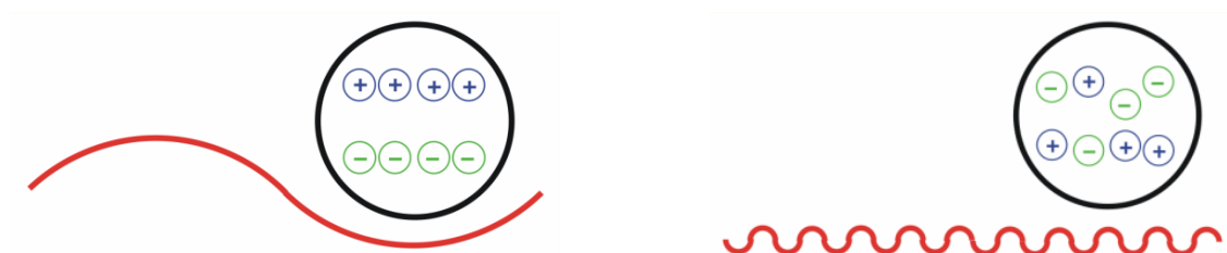
Fig. 3.25 Influence of the laser light wavelength on the induction of dipoles inside the particle: short wavelengths lead to unwished segmentation of the particle.
