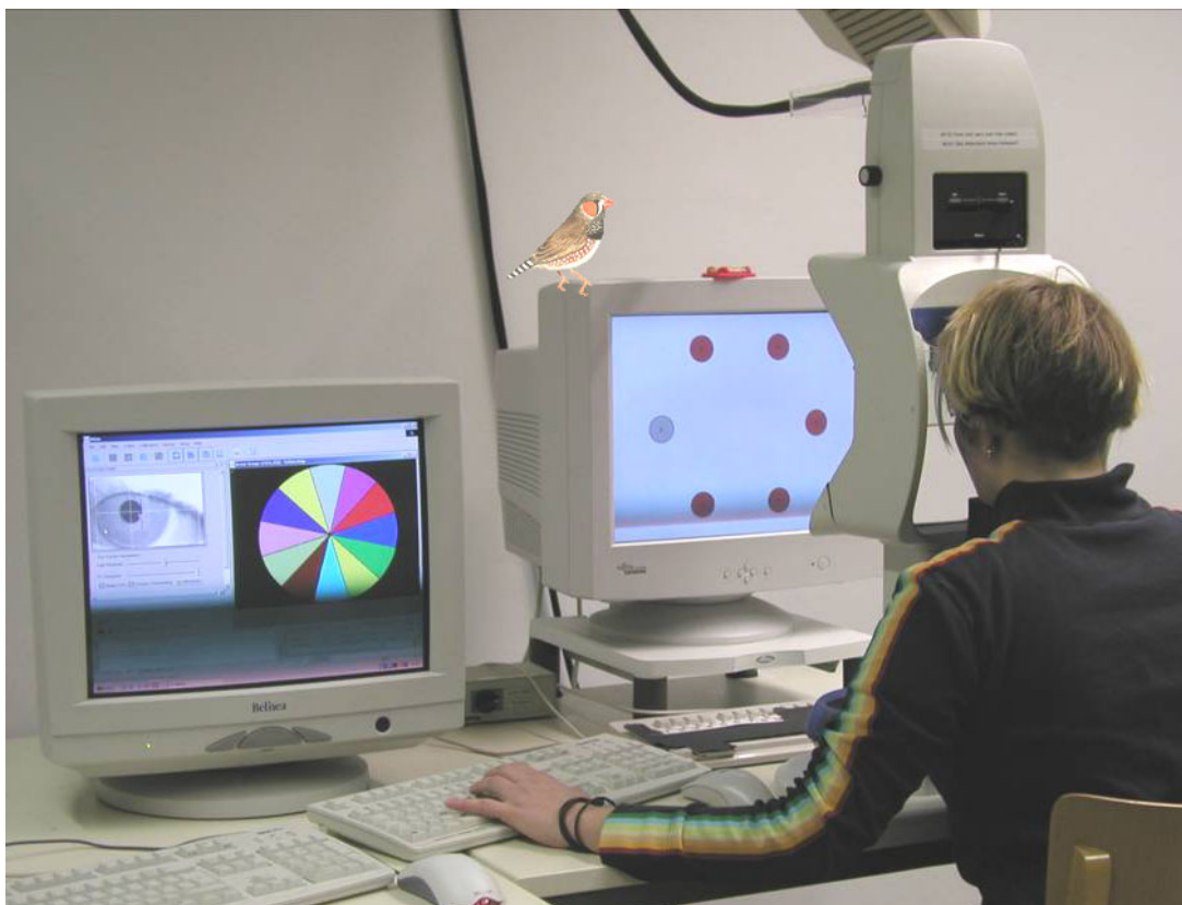
Figure 3: Experimental set-up: infrared eye-tracking system with integrated forehead and chin rest.
