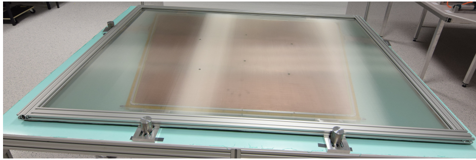
Figure 7.14.: Photograph of the drift panel with mesh during the alignment. Visible are the ears on the drift panel and the cylinders, which are already fixed to the mesh position.
