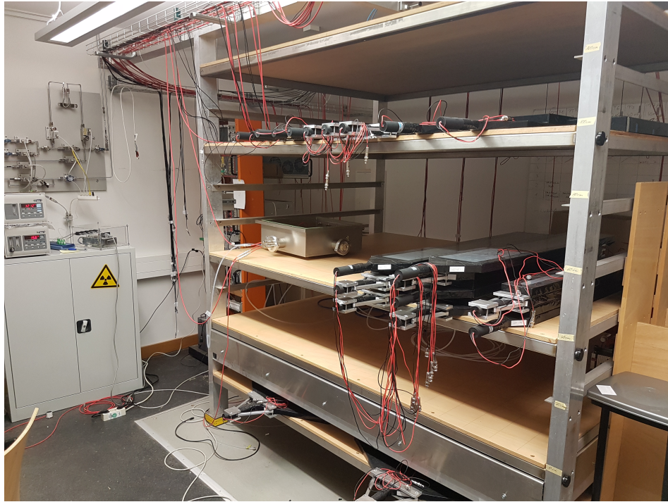
Figure 3.1.: Photograph of the cosmic ray facility. The frame with the scintillators and the pressure chamber can be seen in the center. Behind it is the orange electronics rack. On the left side are the mixing panel and the contamination measurement devices.
