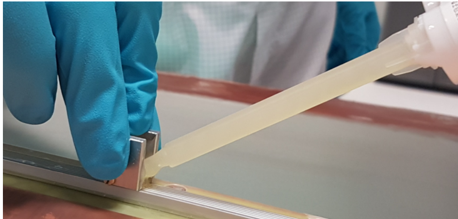
Figure 7.16.: Photograph made during the glue application (first lap). One person is moving the tool steadily along the bar, while another person is applying glue to the front part of the tool.
