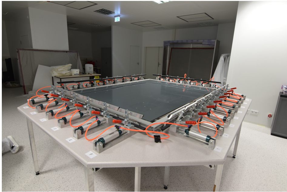
Figure 7.7.: A photograph showing the stretching table. The central plate is in its up position, the transferframe is put onto the clamps, which are arranged and prepared for the mesh transfer.
