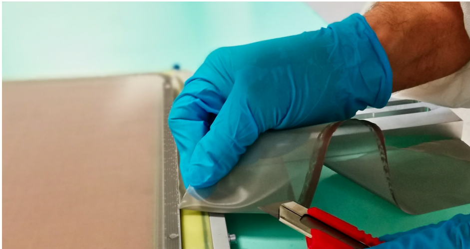
Figure 7.19.: Photograph of the cutting procedure. The mesh has to be taken out carefully to prevent any open wires.
