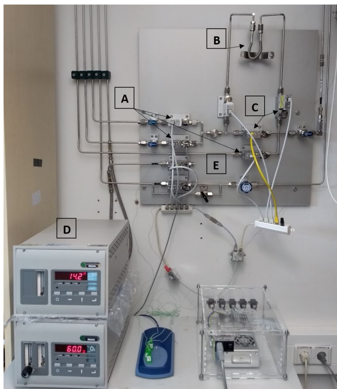
Figure 3.5.: Picture of the mixing panel. A labels the massflow controllers for argon, argon+oxygen and carbon dioxide, B shows the location of the Bubbler, C are the pressure controllers for the bubbler. After the gas passed through the detector, the amount of contaminations is measured in D, before the gas then exits after the pressure controller for the Micromegas at E, from [73]
