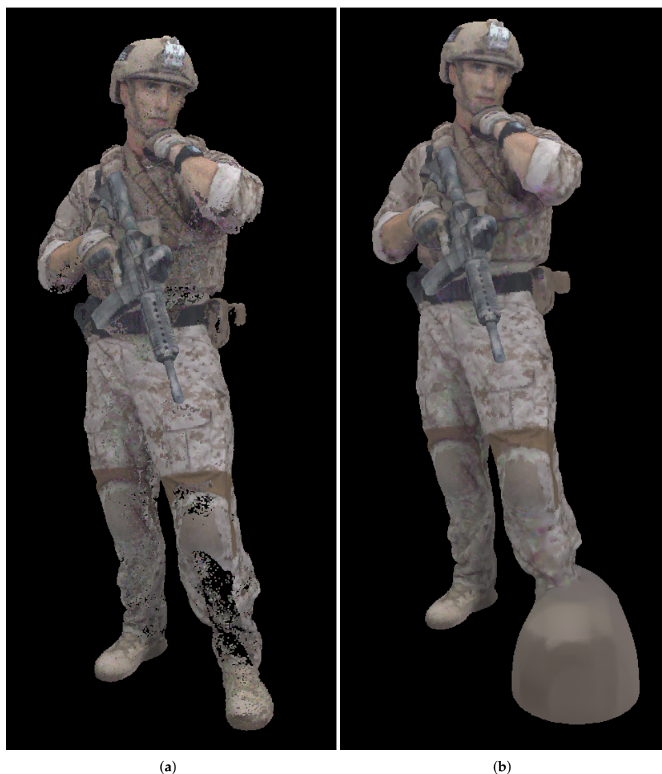
Figure 20. Decompressed point cloud Soldier , “soldier_vox10_0537.ply”-second point cloud used in compression/decompression process, using cylindrical projection with panorama size of 2,000,000 points: (a) before Poisson reconstruction (point size 2 in MeshLab); (b) after Poisson reconstruction (point size 1 in MeshLab).
