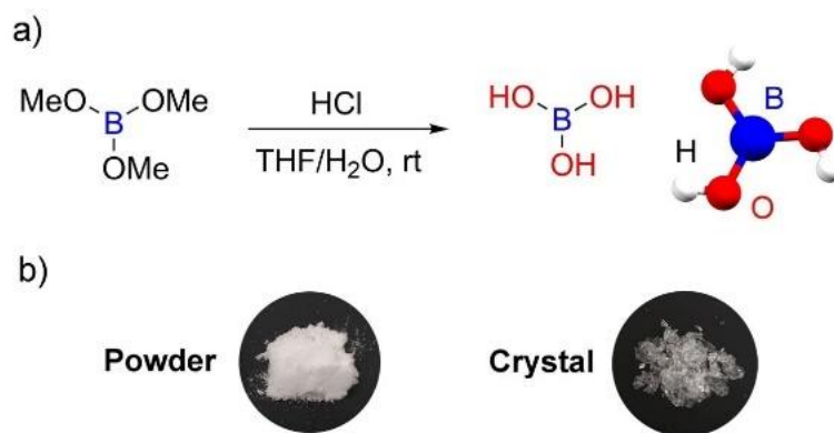
Figure 4-1 a) Synthesis of boric acid from B(OMe)_3 . b) Photographs of BA as a ground powder and as crystals, taken under daylight. The ground powder retains crystallinity.
