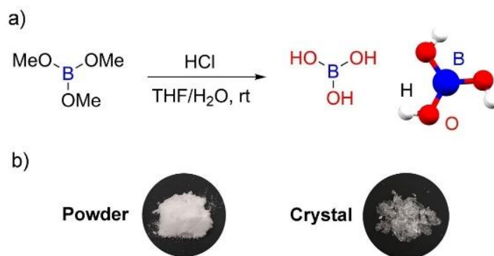
Figure 5-8 a) Synthesis of boric acid from B(OMe)_3 . b) Photographs of BA as a ground powder and as crystals, taken under daylight. The ground powder retains crystallinity.
