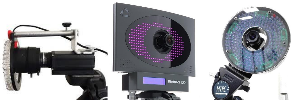
Figure 9: Motion capture cameras. On the left, a BASLER camera, used at UKW for WP-4; in the centre, a BTS SMART-DX camera, used at UKW for WP-1; on the right, a BTS SMART-D camera, used at the LAMB laboratory for WP-2 and WP-3
