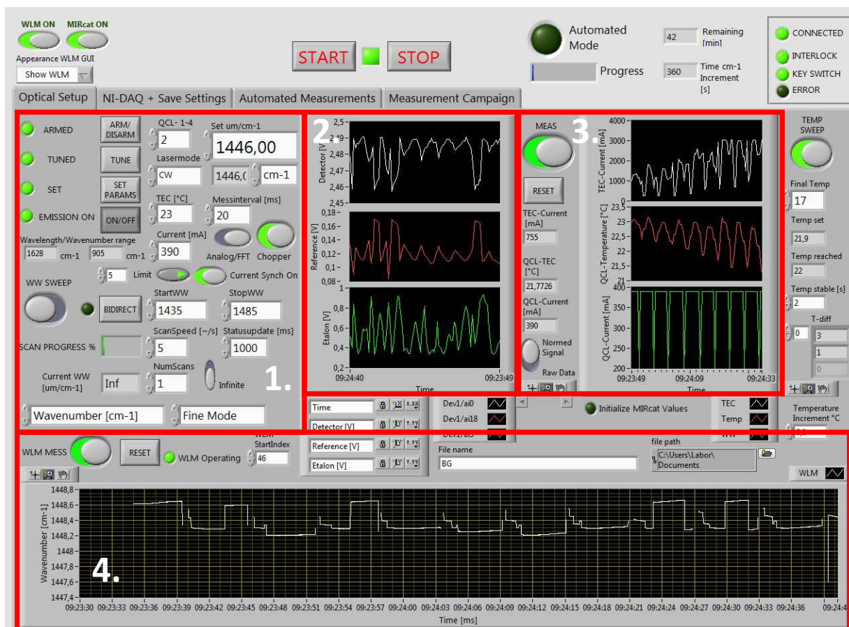
Figure A.2: Screenshot of in LabVIEW developed GUI for operation of the optical setup. The figure shows the GUI during a spectroscopic measurement. Four main parts of the control elements are marked in red rectangles and indicated with respective numbers:
