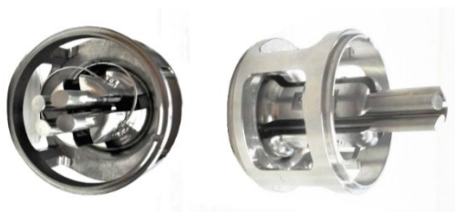
Figure 2 Photographs of a quadrupole used in Sciex mass spectrometers (photo by Jonas Wohlfart)
