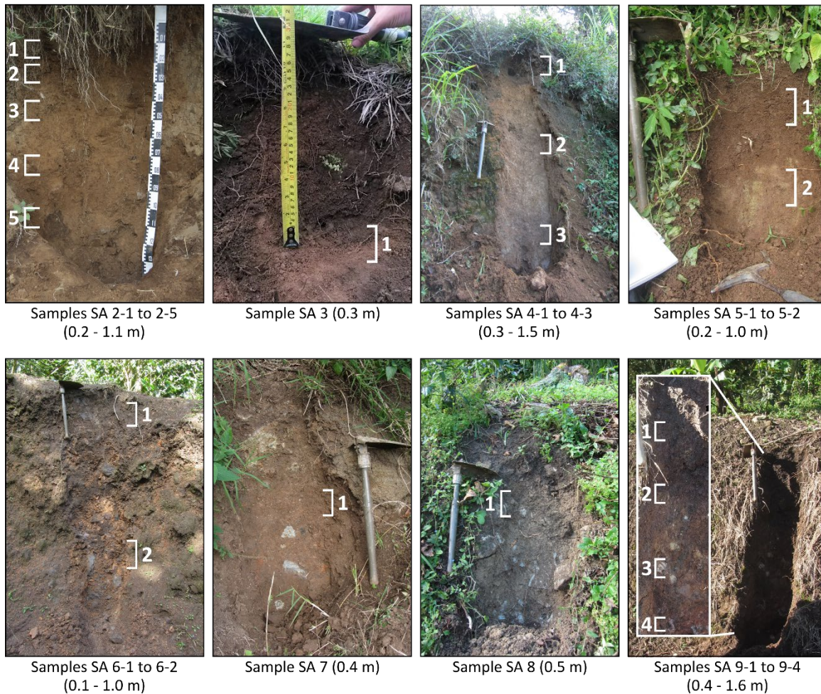
Figure 5-17. Sample locations (SA 2 - SA 9) of the surrounding areas of the Capulín landslide. The sampling areas are marked with white squared brackets. The sampling depths as indicated in the labels are measured from the ground surface. Source: Photographs T. Sprafke (2016).
