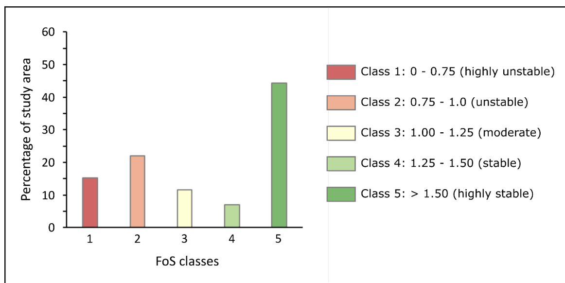
Figure 6-6. Proportion of the stability classes in relation to the study area in percentage for the simple SAFETYFACTOR map. Susceptibility classification modified after Teixeira et al. (2015). Source: Own illustration.
