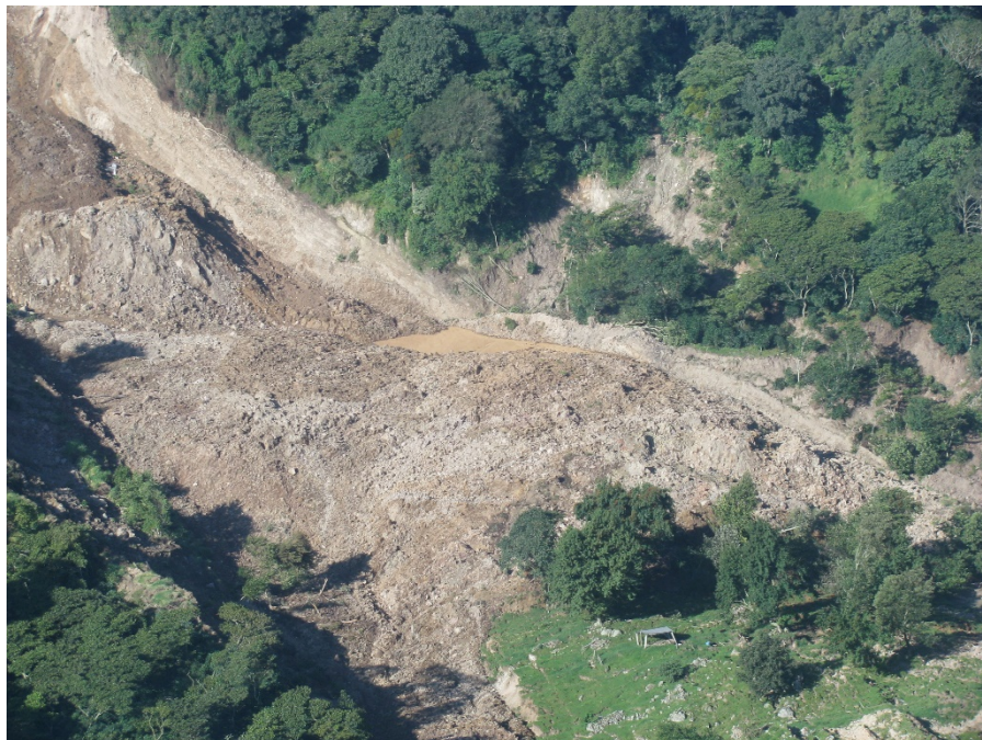
Figure 7-12. Area of high distortion between the two slide blocks of the Capulín landslide. Upper part of the lower slide block, including intact trees, is at the lower right corner of the photograph. Source: Photographs: S. Rodríguez Elizarrarás, 2013.
