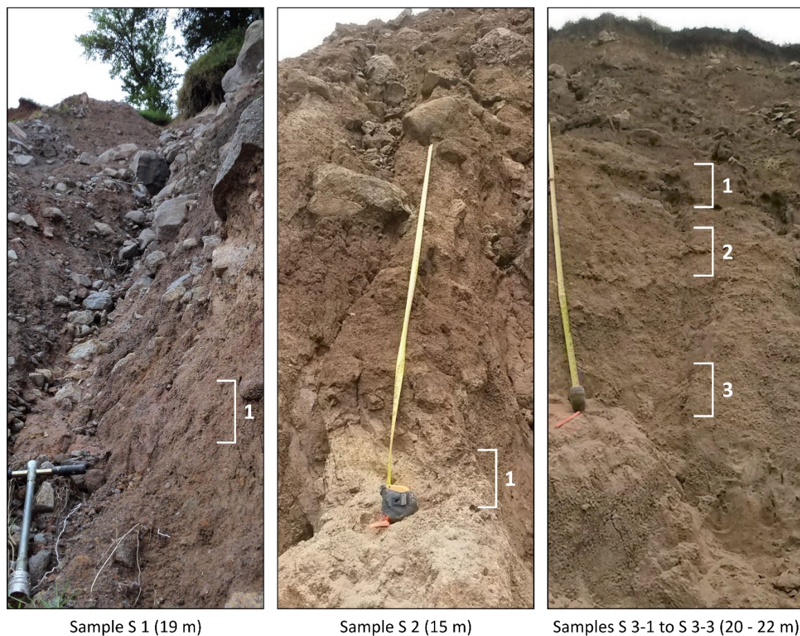
Figure 5-3. Location of the scarp samples (Capulín landslide). S 1 and S 2 are located in the center of the scarp, S 3 is located in the western part. The sampling areas are marked with white squared brackets. The sampling depths as indicated in the labels are measured from the top of the scarp. Source: Own photographs (2018).
