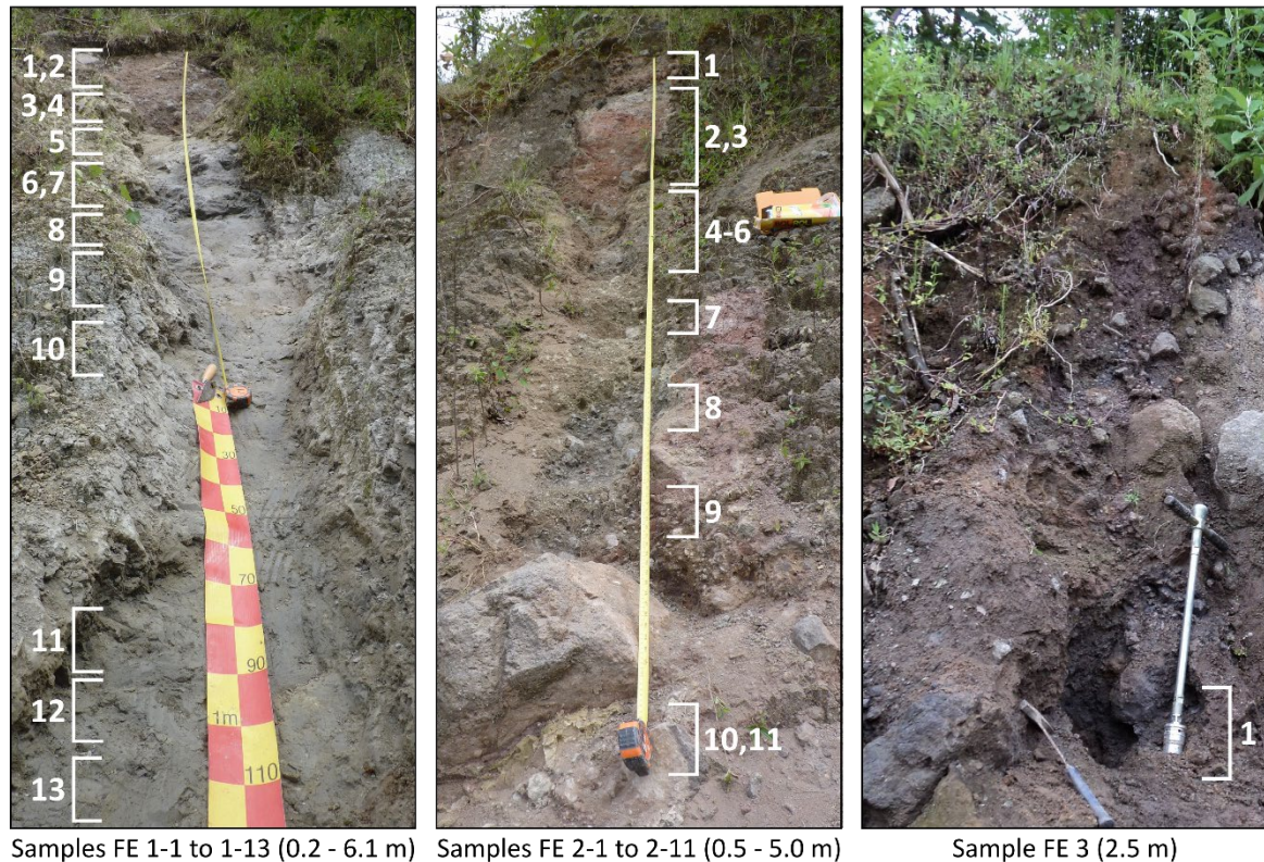
Figure 5-7. Photos of the sample locations of the eastern flank (Capulín landslide). The sampling areas are marked with white squared brackets. The sampling depths as indicated in the labels are measured from the ground surface. Source: Own photographs (2018).
