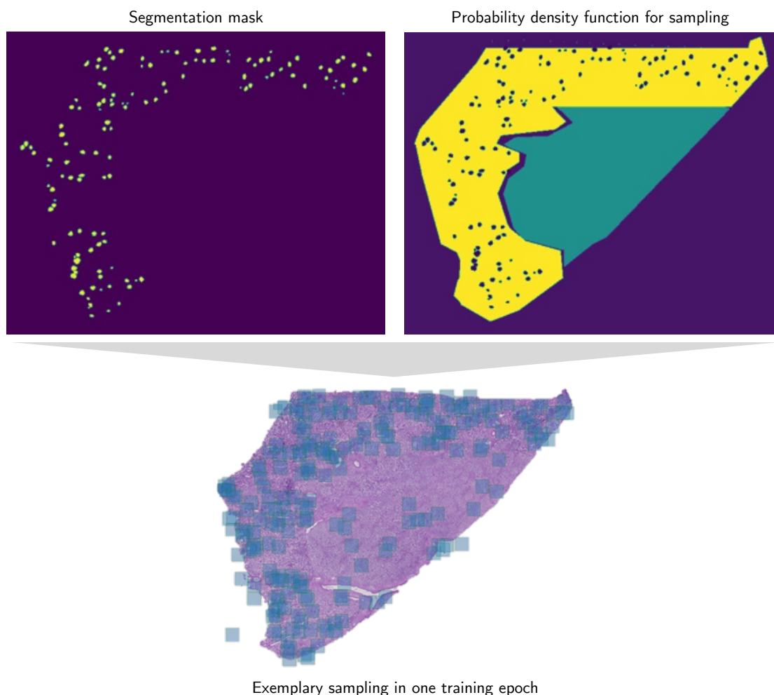
Figure 2.5.3: Exemplary sampling of 512 \times 512 pixel tiles from image “0486052bb” during one training epoch, showing the segmentation masks of the annotated glomeruli (top left) and anatomical region probabilities (top right). The colors indicate the sampling probabilities, from low (purple) to high (yellow). The sampled tiles (squares) during one training epoch are depicted at the bottom.
