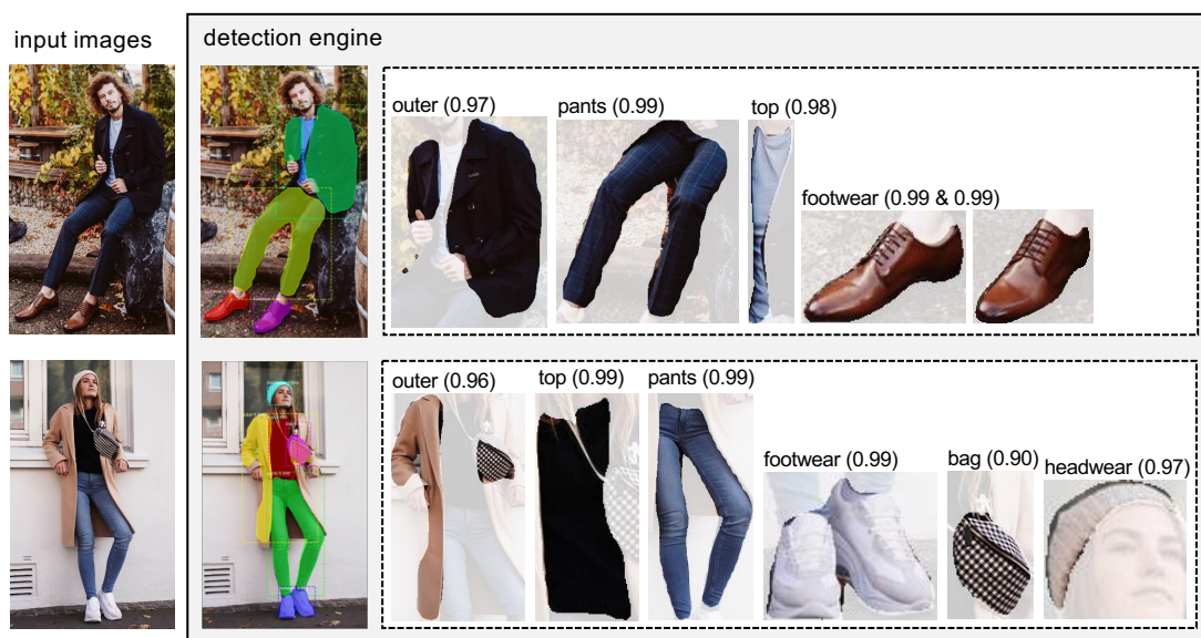
Figure 2.3.5: Demonstration of the detection engine (example images taken from zalando.com). The detected garment class names and probabilities are shown in the white box.
