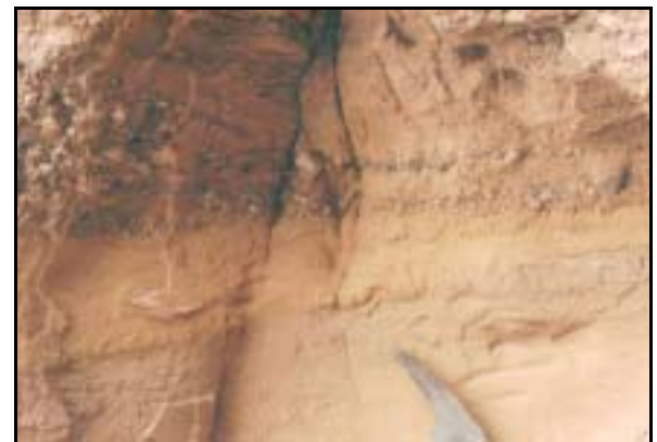
Fig. 29: Detail of lithofacies F. Note the internal structures of cross lamination and local intercalations of pebble-sized material.
