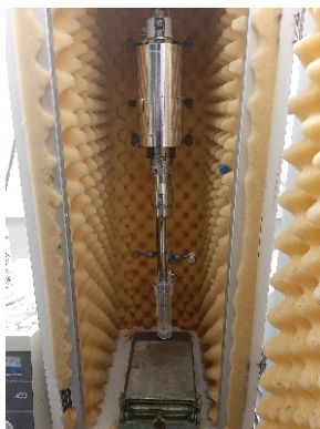
Figure 3.4: Image of the sonication setup. The falcon tube is submerged in an ice bath during operation, to ensure proper cooling.
