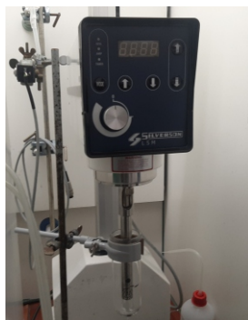
Figure 3.3: Image of the shear mixing setup. During normal operation the glass flask is submerged in a water bath to provide sufficient cooling.
