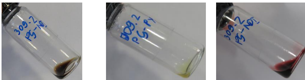
Figure 4.2.3.3-1: Solutions of P(G-co-NDI) (left), P(G-co-Pyr) (middle) and mixture of both (right) in water with G:Pyr = 57:3 and G:NDI = 54:6 with 10 wt-% polymer in total.
