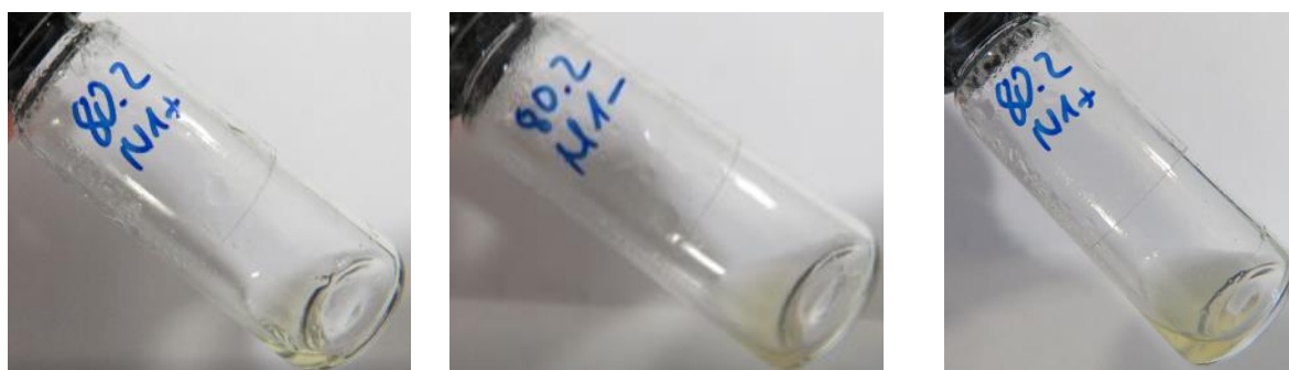
Figure 4.2.2.3: Solution of P(G-co-Im) (left), P(G-co-POH) (middle) and equimolar mixture of both (right) in PBS with G:Im = 48:11.6 and G:POH = 48:12 and 10 wt-% polymer in total.
