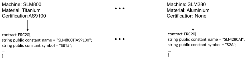
Figure 7.4: Each Combination of Machine, Material and Certification Corresponds to a Unique Token
