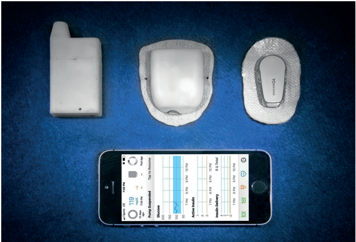
Figure 12.1: Loop System Components
