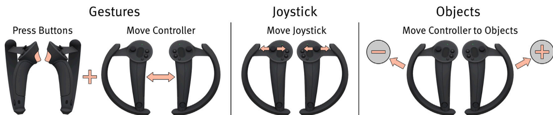
FIGURE 5 The figure sketches the three body weight modification methods we used for our evaluation: Gestures (left), Joystick (center), and Objects (right).
