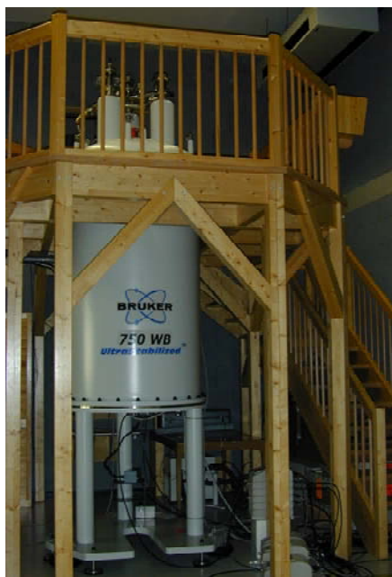
Figure 3.1: Avance 750. Magnet and preamplifiers of the four channels are shown (bottom right).
