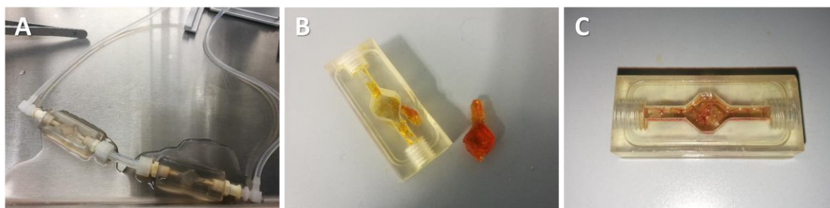
Figure 80: Problems of the usage of Gelatin/Ruthenium hydrogels for dynamically cultivated bi-layered artery models. A After a certain culture period, strong leakage was observed in the models. B Gelatin/Ruthenium hydrogels were sticking to the chamber walls, destroying the models during removal from the chamber. C Leakage of the perfusion system furthermore destroyed the models by dehydration.
