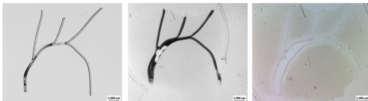
Figure 96: Proof-of-concept for the generation of an aortic artery model . A Printed POx scaffold in the shape of an aorta. B Scaffold embedded in 8% mTG-hydrogel before dissolution of the polymer and C after dissolution of the polymer, creating an aortic-like channel structure in the hydrogel.
