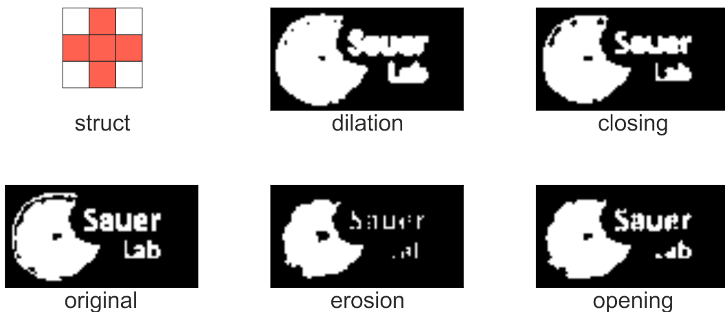
Figure 16: Morphological operations The Structural element for the used morphological operations. original image, erosion, dilation, closing and opening.
