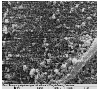
Abb. 5.121: REM; Vergr. 10000x; DATEM/3,0% SIPER NAT ® 22S; Turbula ® ; 42 UpM; 30 min
