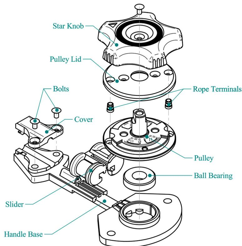
**Figure 2.** Exploded view of the control handle with its main elements.
