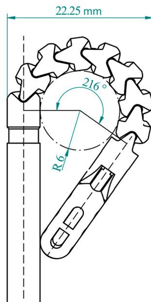
**Figure 1.** Image of the instrument's distal tip at the maximal bending angle with annotated dimensions.
