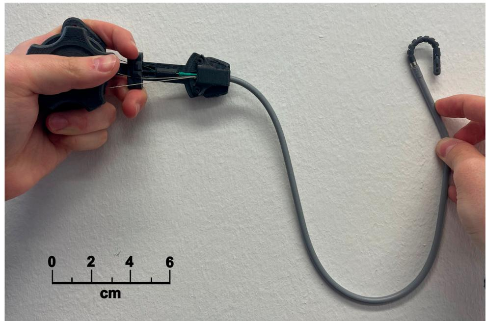
**Figure 3.** Image of the prototype developed for the study. The flexible shaft and the distal tip are bent, showing the degree of the instrument's flexibility. The depicted prototype is 50 cm long.
