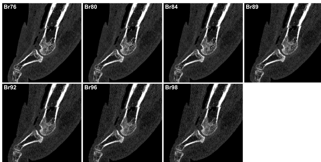
Figure 2. Image quality. Image quality associated with sharp non-UHR and all six available UHR kernels on representative sagittal slices depicting a midtarsal fracture. Importantly, sharper UHR kernels induced amplified image noise, which is particularly visible in soft tissue areas. Elevated noise levels were found to impair osseous assessability to a certain extent.
