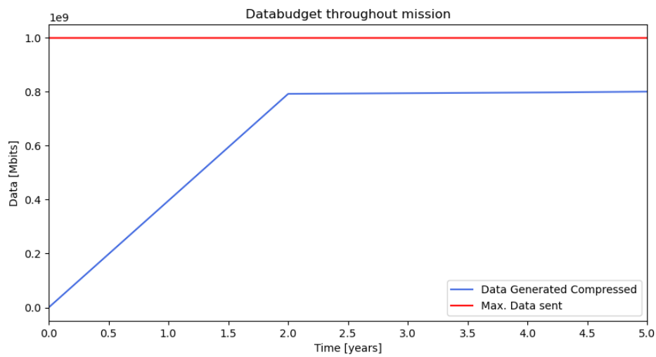
Figure 16.9: Simulation of mission data budget. Operation times: SAR for two years (0-2), all other instruments for two years (2-4) and the experiment for search for life in Venus' atmosphere for one year (4-5). Max. possible data amount that can be transmitted during the overall mission is displayed.
