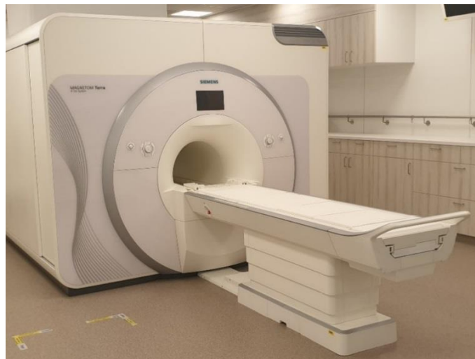
Figure 7. 7T Terra whole-body MR scanner for conducting in vivo experiments in human volunteers, patients, and large animals. The MR scanner, which was installed at the Comprehensive Heart Failure Center (CHFC) as part of the University Hospital Würzburg, facilitated state-of-the-art technologies such as parallel signal transmission.
