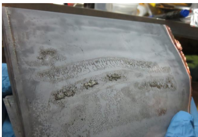
Figure S 2. Photograph of anode facing a cathode with ripples. Metallic lithium plating on the surface of the anode is visible.
