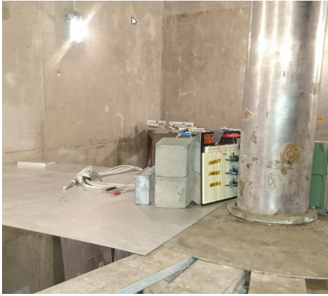
(A) Test setup with a Cobalt-60 source and the DUTs
