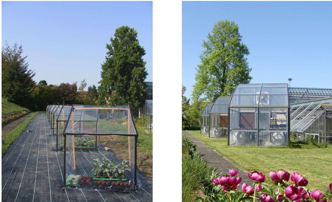
Fig. 1.1.3 Different experimental designs. Twelve filter tents (left) covered with either UV-B and UV-A including (+UV, Teflon foil) or excluding (-UV, Lee 226 foil) filter foils and three greenhouses (right) covered with innovative materials, transmitting either high (80%, ETFE foil), medium (23%, MM glass) or low (4%, float glass) levels of UV-B (for filter qualities see Fig. 1.1.4).
