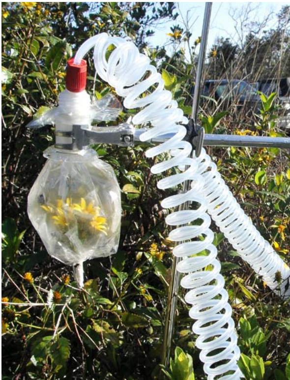
Fig. 2 Odour source that supplies the arena of the olfactometer with floral scent.
