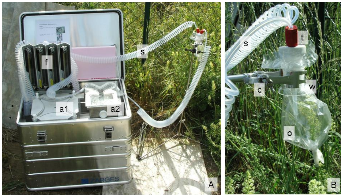
Fig. 1 Mobile Olfactometer (A) and scent application (B), including the four field arena (a1), Y-shaped arena (a2), flowmeters (f), spiral Teflon tubes for air transport (s), oven bag (o), laboratory clamp (c), cut washing flask top (w) and the Teflon washing flask topping (t).
