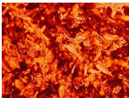
Figure 15. POM textures of ( P )- 4b after cooling down ( 0.1\text{ }^{\circ}\text{C min}^{-1} ) up to 96\text{ }^{\circ}\text{C} from the isotropic phase.
