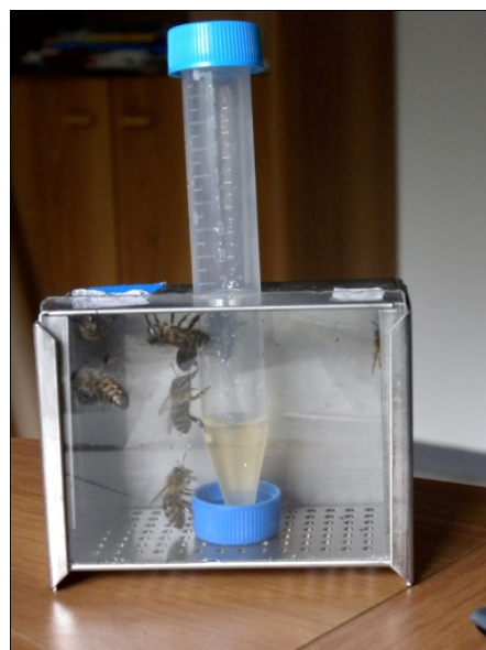
Figure 20: Stainless steel cage with feeding tube used in the toxicity cage tests.
