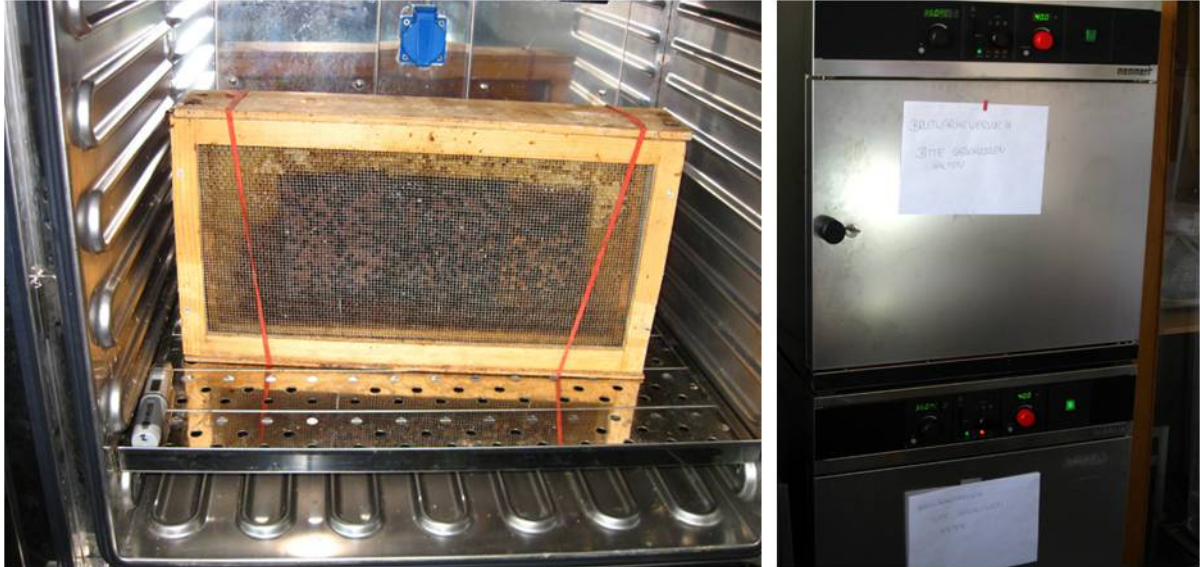
Figure 11: left: Pieces of brood combs from different hives embedded into a honey comb and framed in a cage to keep the freshly hatched bees confined on the comb. right: Memmert IPP 500 incubator used to store the combs.
