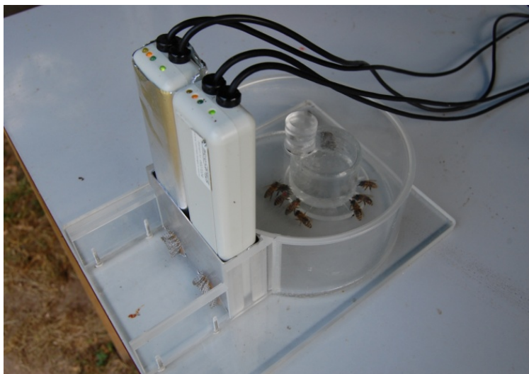
Figure 24: Feeder chamber enabling automatic registration of RFID tagged bees entering and leaving the food source.
