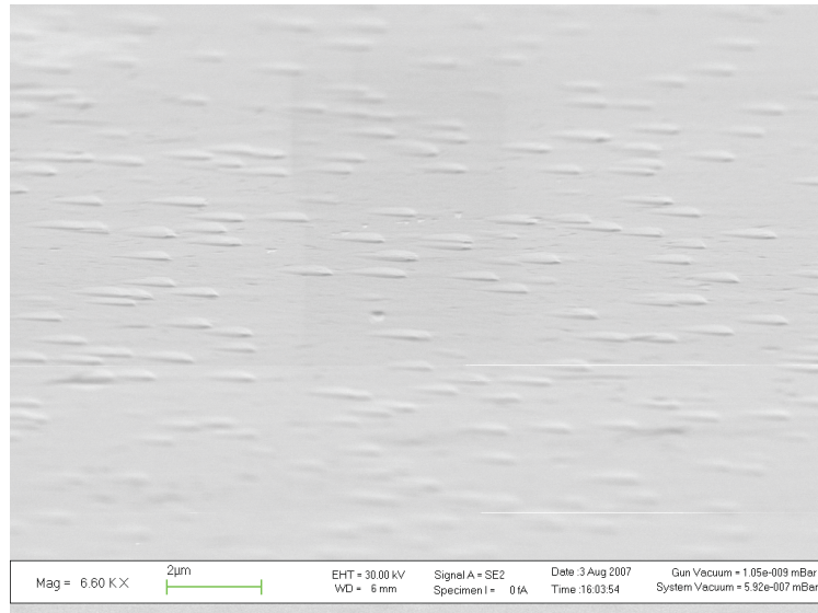
Figure 7.20.: SEM picture from the sample with 20nm NiMnSb. The triangle defects are distributed randomly over the sample but all aligned in the same direction.
