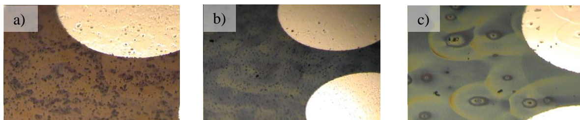
Figure 39. Images obtained under optical microscope of solar cells built with a) HB255 (75wt% PC 61 BM, chloroform); b) HB101 (75wt% PC 61 BM, chlorobenzene with 20% pyridine) and c) MD356 (75wt% PC 61 BM, chloroform). The light area represents the electrode material, the dark area the active layer between the single cells on one substrate.
