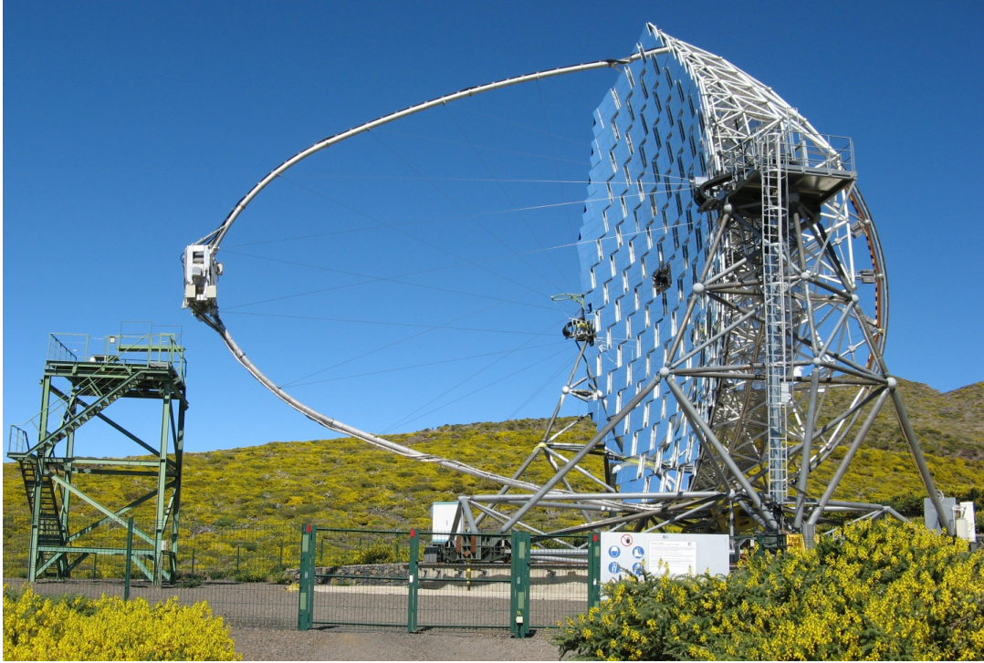
Figure 4.6: MAGIC-I in July 2007. Each the mirror diameter as well as the distance between the camera and the mirror centre amount to 17 m. The tessellated structure of the mirror as well as the hole at the centre housing several sub systems is clearly visible.
