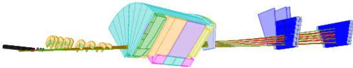
Figure 5.15.: Schematic view of the ATLAS detector elements passed by muons with transverse momenta of 10 GeV (green) and 15 GeV (red) when they are bended in the toroid magnetic field. The pseudorapidity of the tracks is in the range [2.5; 2.7] in steps of 0.05.
