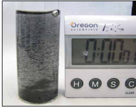
Figure 12: Large agglomerates of 500 nm (primary size) magnetite nanoparticles immediately form due to mutual magnetic attraction after shaking up magnetically extracted particles again in solution.
