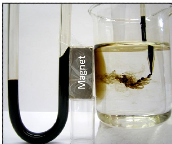
Figure 36: A water miscible ferrofluid ( sol ), i.e., an aqueous magnetic nanoparticle dispersion ( c = 23 \text{ g/l} , synthesis and discussion in chapters 4.1.2.3 and 4.1.3.1 ) is attracted by a magnet (left). Added to water, it is attracted by the magnet as a cloud (right). This might in principle be used as a “comb” to clean water from contaminants as the miscibility with contaminated water might promote the adsorption of hazardous substances to the nanoparticles in the ferrofluid. Sol-liquid separation can be achieved; however, solid-liquid separation of individual magnetic nanoparticles does not seem to be possible.
