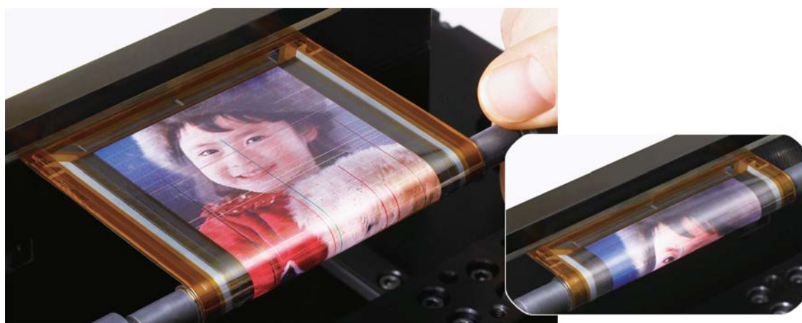
Figure 1. The first flexible OLED display that can be rolled up on a pen while still displaying the video was presented in May 2010 by Sony. Reprinted with permission from ref. 6. Copyright 2011, Society for Information Display.
