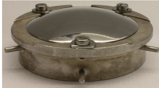
Figure A.6: A mirror on a Molybdenum block which can be inserted into the UHV growth chamber. The tool offers a front view at the effusion cells and its cell shutters.
