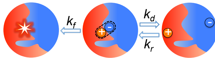
Figure 2.3.: Schematic description of the possible processes determining the dissociation probability P of polaron pairs (see Eq. (2.1)). The desired dissociation takes place with the dissociation rate k_d . These free charge carriers can recombine again with a certain rate k_r into the bound polaron pair state, which can once more be dissolved or decays with the rate k_f .
