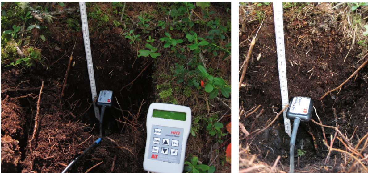
Figure 2.6: Humus moisture and temperature measurements using the WET sensor.
