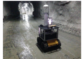
Figure 3.13: Husky A200 robot with Riegl VZ-400 inside the mine by Leung et al.
