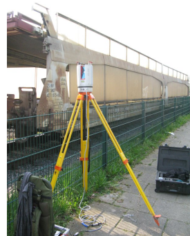
Figure 3.16: The Riegl VZ-400 laser scanner set up next to the train wagon.
