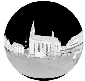
Figure 2.7: The scan from Figure 2.6 as reflectance image on a perfect sphere surface in the same orientation.
