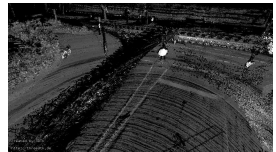
Figure 1: The same car multiple times from the KITTI dataset due to the same car being present in multiple scans at different positions in a mobile mapping scenario
